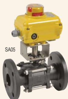
765 XS - Electric actuated carbon steel ball valve A216WCB body - CF8M ball - TS: -25°C/+220°C - ⚠ Steam use: PS: 15 bar / TS: +200°C.
