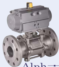
711 XS - Pneumatic actuated stainless steel ball valve Direct mounting - CF8M body & ball - TS: -30°C/+218°C.
